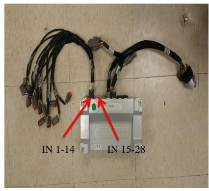
Leads go to the blockage sensors. Note: don't need the voltage adapter with the Apollo.
