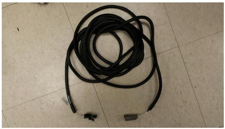
This harness connects to the main tillage harness on the whisker connector. It will then run to the front to the solenoid on the 3320/3720 and to the proximity switch on the 5810/8910. Note: with the Apollo system you will no longer need the relay.
