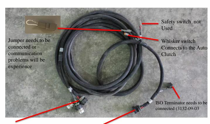
Connectors hook to the rear plate of the Leading tank.
