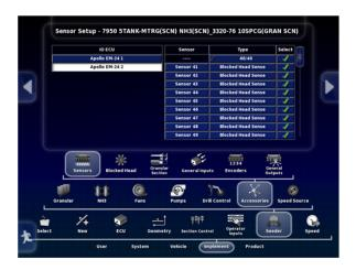
49. If configured with Blockage go to Implement/Seeder/Accessories/Blocked Head and select enabled. Settings should be preloaded from factory profile.
