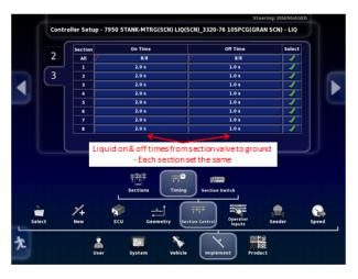
35. Under the Section Switch tab enable Virtual Section Switches if you want the ability to override ASC by manually shutting off sections. For the liquid/NH3 boom match the # of switches to the # of sections.
