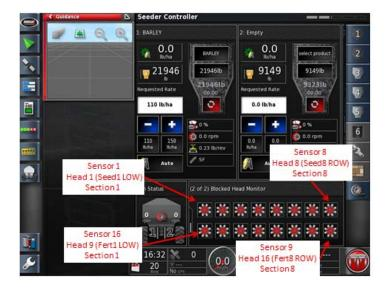
52. Refer to the figure below showing how the blockage sensors are wired from the factory and should be assigned to show up correctly on the screen.
