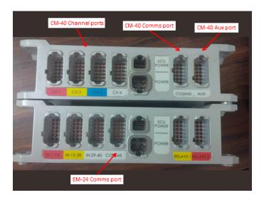
18. Under Implement/ECU/Add/Replace ECU select the tab under the Status column for the 1<sup>st</sup> CM-40 ECU on the list. Select Replace CM-40 and accept.
