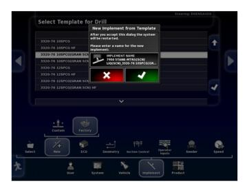
17. The ECU's need to be detected one at a time, starting with the master CM-40 ECU, for each new implement profile. To do this, all the Comms connectors on the ECU's need to be unplugged except the master CM-40 ECU. (If there is more than one CM-40 ECU on the tank the master should be the 1<sup>st</sup> one bolted to the tank. It will have all 4 channels connected and a harness connected in the AUX port.)
