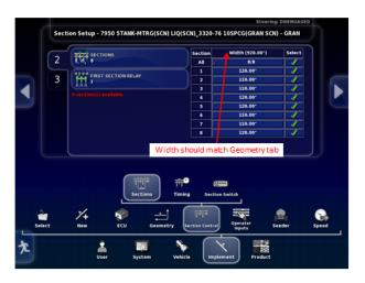
33. If configured with liquid/NH3 set up # of sections and the section widths for that boom.
