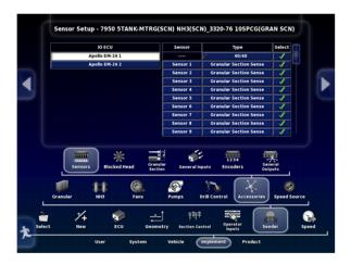
48. If configured with Blockage the 2<sup>nd</sup> EM-24 ECU (1<sup>st</sup> EM-24 if no ASC) should have the sensor Type column preset to Blocked Head Sense.
