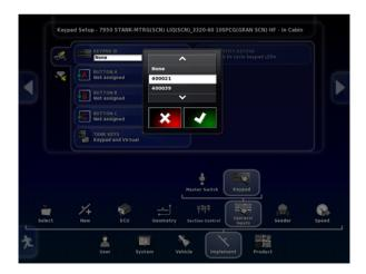
37. You can confirm you have the right keypad assigned in the cab as the LED lights will stop flashing. There is also an Identify Keypad button that changes the flash sequence to confirm you have the right one selected for the appropriate location.
