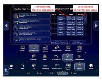
51. Refer to the figure below showing how the blockage sensors show up on the screen if assigned as described from factory settings.
