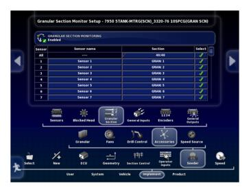
54. Under Implement/Seeder/Speed Source select the Speed Source you will be using. If using GPS you can set a Fallback Type to keep seeding if the GPS signal drops out.
