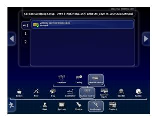
36. Under Implement/Operator Inputs/Keypad select the Keypad ID for the in-cab keypad & on-frame keypad.
