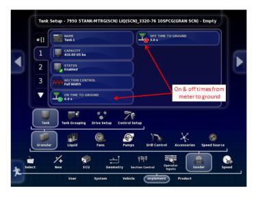
43. Under Implement/Seeder/Granular/Drive Setup set the Metering Auger type for each tank.
