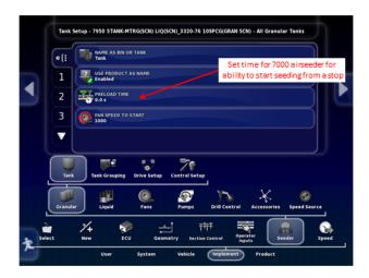
41. Set the on & off timing for each tank. On a sectional boom this is the time from the meter to the section valve. This can be 1 sec on & off for a tow-behind configuration. This should be measured for a leading configuration since it may vary more significantly.
