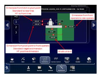
32. The Implement /Section Control tab only appears if configured with granular or liquid/NH3 ASC. On the Sections tab for the granular boom, the total width should match the width on the Geometry tab for that boom.
