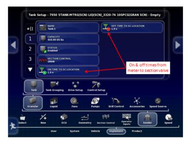
42. It is important to note that for a full width configuration, or if you change the tanks to be controlled by the full width boom, that the wording for this timing changes to Time to Ground. This timing needs to be changed to the time from the meter to the ground.
