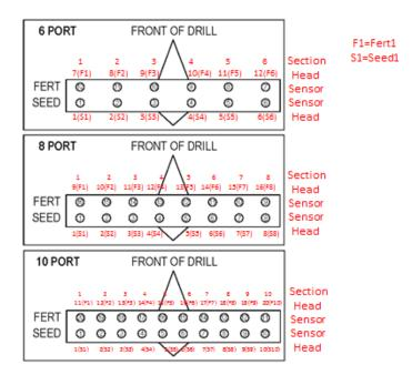
53. Under Implement/Seeder/Accessories/Granular Section there should be a section pre-assigned for each sensor in the same order.
