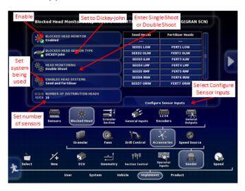
50. Press Configure Sensor Inputs. Sensors should be pre-assigned from factory profile. If configured with granular ASC then the sensors are also assigned to the corresponding section.
