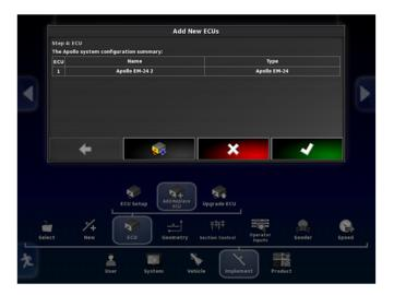
30. Once all ECU's are detected there should be firmware versions listed for each ECU indicating that the system is communicating with each.
