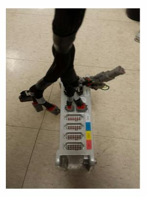
One Master ECU configured for 4 tank metering. No sectional control or NH3 or liquid
