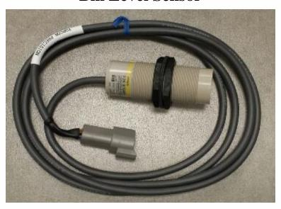
Each air seeder compartment that has a metering auger contains a single bin level sensor installed near the bottom. The sensor will trigger an alarm when there is no product in front of it.
