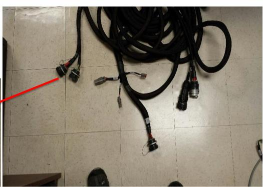
Note: This harness needs to be in place if there is no Blockage or sectional control on the drill
