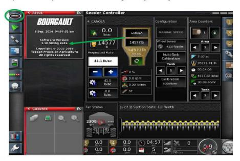
11. On main screen, click the Bourgault button in the top left hand corner. Ensure that the software version shown is correct. (3.18.513bg)
