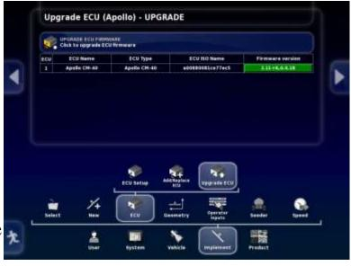
You may have to shut down/unplug ISO connector at the back of the tractor to get ECU information to upload.
