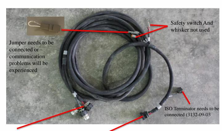
Connectors hook to the rear plate of the tillage machine.
