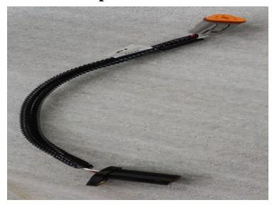
There are speed sensors in several locations on the air seeder. These include fan speed, ground speed, and metering auger speed. All of these sensors are proximity style and send a signal to the ECU.
