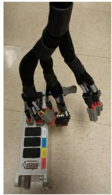
One Master ECU configured for 4 tank metering. No sectional control or NH3 or liquid
