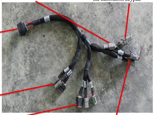
Three connection Comms, power A, and Power B hook to the Master ECU.
