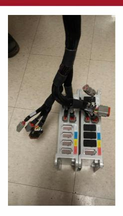
If tank has five tank metering a second Master (CM-40) needs to be added in. Or if the tank has four tank meters and NH3 or liquid.
