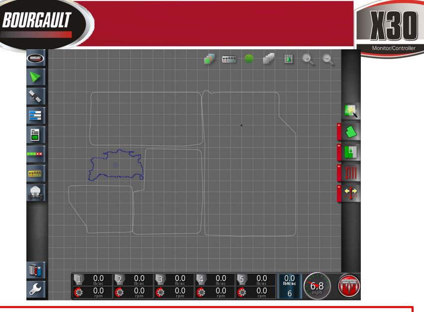
The above screen shows 5 different Field Boundaries, the Blue on is the one that is currently loaded and the light grey ones are the other fields in the general location.
