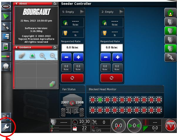
Enter SETUP by touching the wrench located in the lower left corner of the operation screen of the X30.
