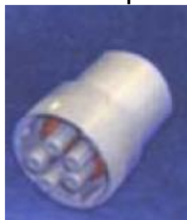
Figure 9 Existing aux. switch plug on case harness
