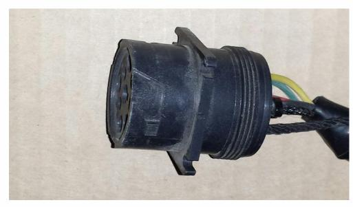
The Deutsch diagnostic connector show above must be removed from the Deere harness and a 3132-94-40 DT04-4P connector kit installed as shown in the right hand image. (the following page details the pin locations of the DT04-4P Deutsch connector)
