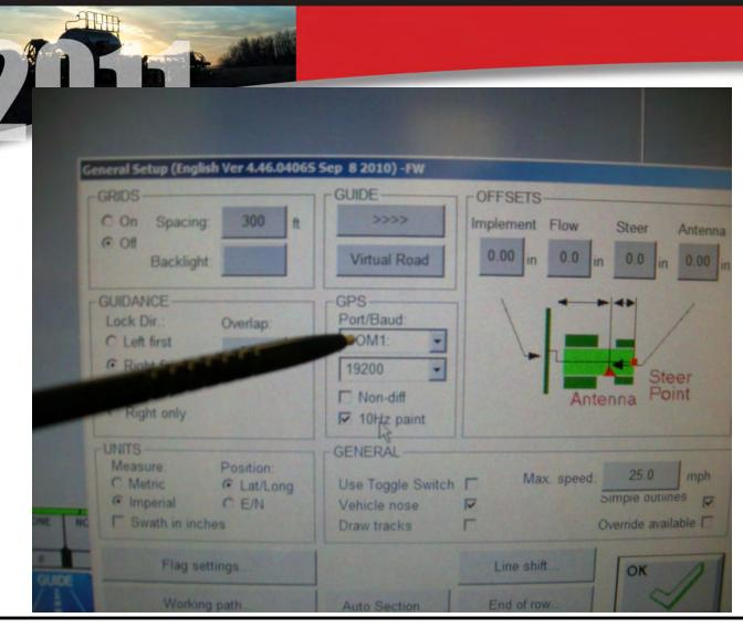
Always select COM1 for guidance which should be where the serial cable from the Greenstar II is connected to at the back of the X20.
