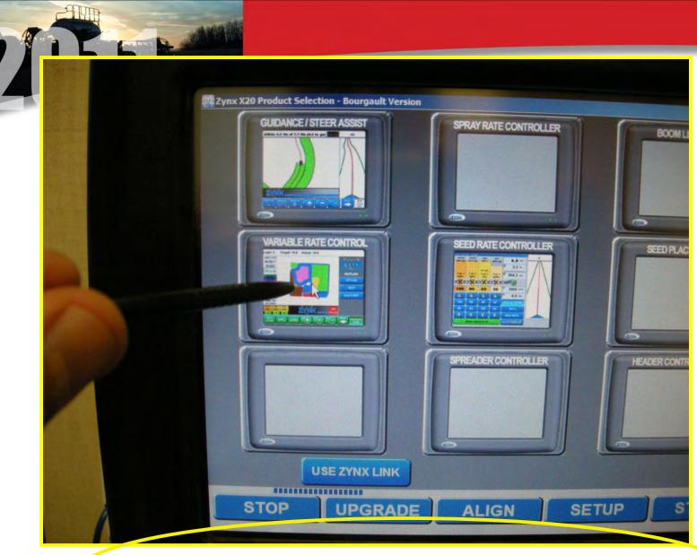
Select Guidance/Steer, Variable Rate Control and Seed Rate Control when starting the X20.
