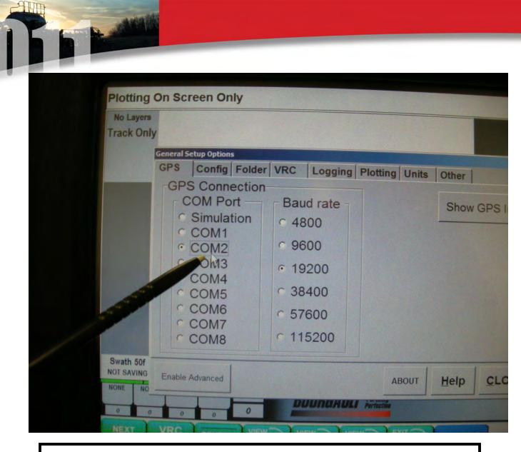
Select COM2 to match where the Maplink serial cable is connected to on the back of the X20
