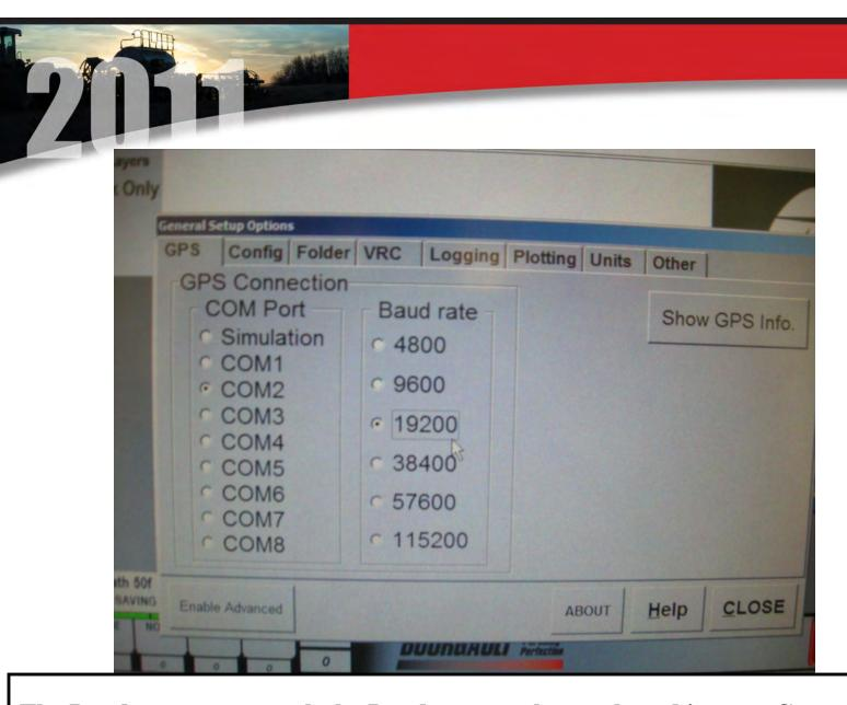
The Baud rate must match the Baud rate you have selected in your Greenstar II. It can be either 19200 or 38400, the picture above shows that 19200 is selected.
