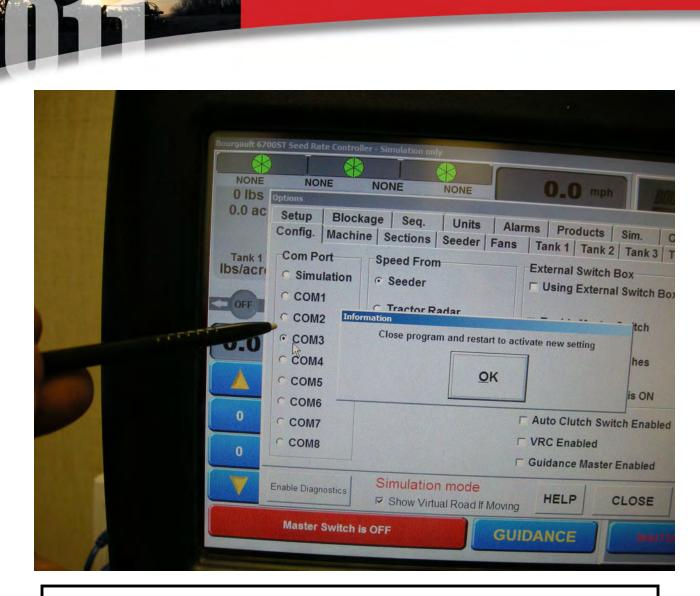
Select Com3 which matches the Com port the SRC serial cable is connected to at the back of the X20.
