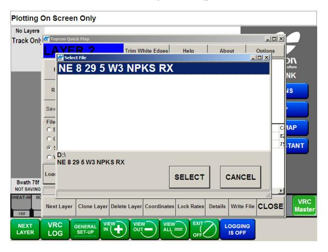
You will have to repeat the process of selecting the map and picking the product for each tank that has product in it. If you are not using all of the tanks you must enter Cloned Layers.
