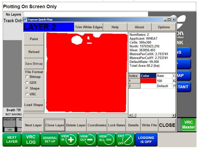
Press Load Shape again to enter Layer 3 and so on till all of the layers are set up
