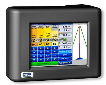
ZYNX Monitor / Control System requires specific sensors and harnesses, including an ECU module located on the air seeder frame.
