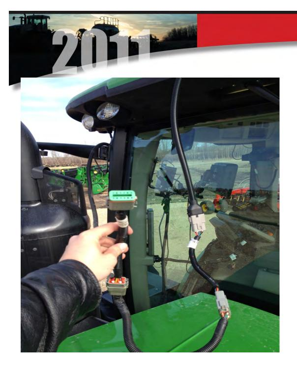
CONNECT MALE/MALE CONNECTOR PF80722 INTO THE FEMALE CONNECTOR ON THE PF90350 GPS SPEED CABLE
