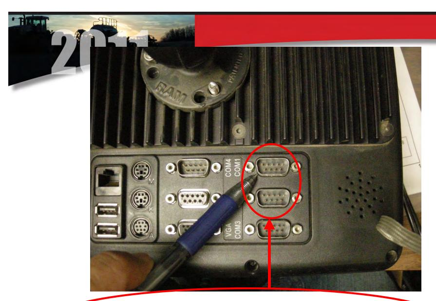
You must plug the serial port Y cable (3131-07) that comes from the Greenstar II into COM1 and COM2 located on the X20 here.
