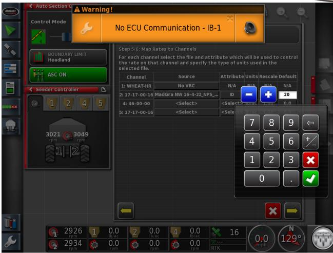
Always enter a Default rate for VRC tanks, failure to do so would cause the rate to go to "0" in the event that you loose GPS.
