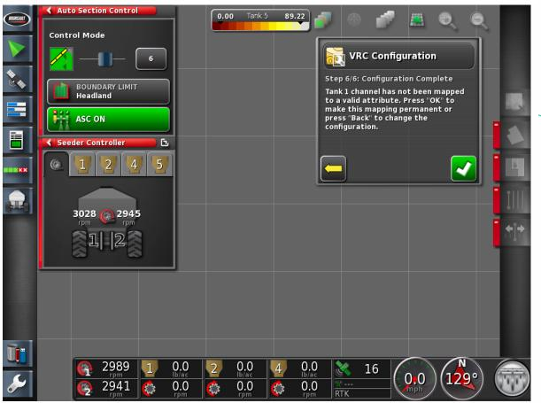
The Green check mark completes the VRC map loading process
