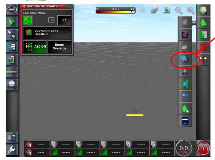
Select this tab to load a Boundary into the X30
