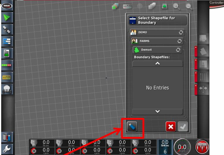
Select the USB tab to load a shape file from a USB memory device.
