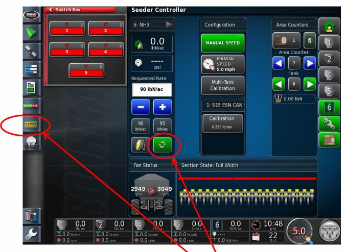
Go to the Running screen, select the Virtual Switchbox on the LH side of the screen. Turn on the clutch for the NH3/Liquid as well.
