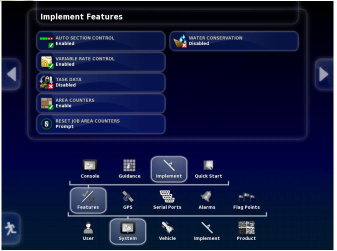
Enter Setup/System/Features/Implement then enable Auto Section Control.
