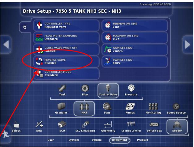
Reverse Valve should be disabled for this test. (after test are completed the valve direction should be verified)
