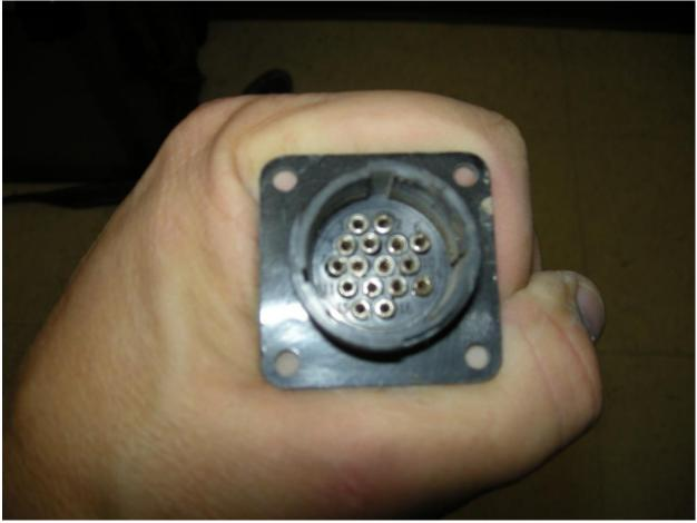
With a voltmeter set to read voltage put the negative lead on pin 4 and the positive lead on pin 3 of the 3151-00 harness. Have someone turn on the NH3/Liquid clutch and you should see +12 volts. (this will be the same for both 2 Valve systems and Fast Valve systems)
