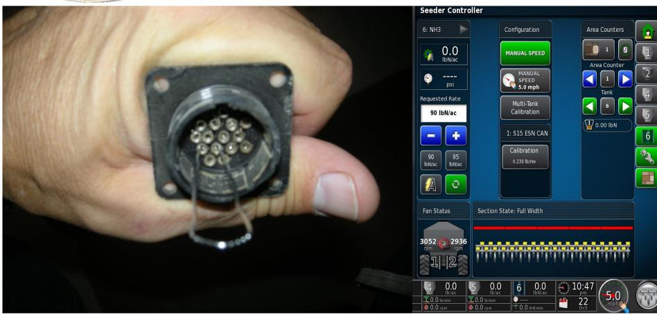
Go to the Running screen to view Area and with a small wire such as a paper clip short between pin 11 (GND) and pin 13 (signal) of the 3151-00 harness. Each pulse will register 1 lb of product in the area counter.
