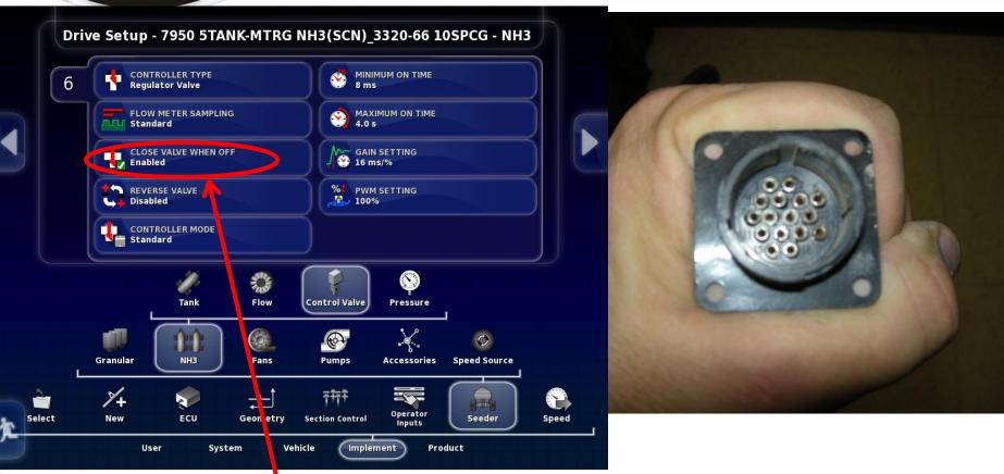
If the Close Valve When Off is selected the voltage will show -12Volts when the NH3/Liquid clutch is turned off and the Negative lead is on pin 4 and Positive lead on pin 3. (This is the normal configuration of a Fast Valve system)
