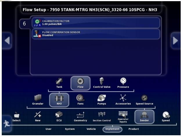
Enter Setup/Implement/Seeder/NH3or Liquid/Flow. Record the existing Calibration Factor for future reference and enter a Calibration Factor of 1.
