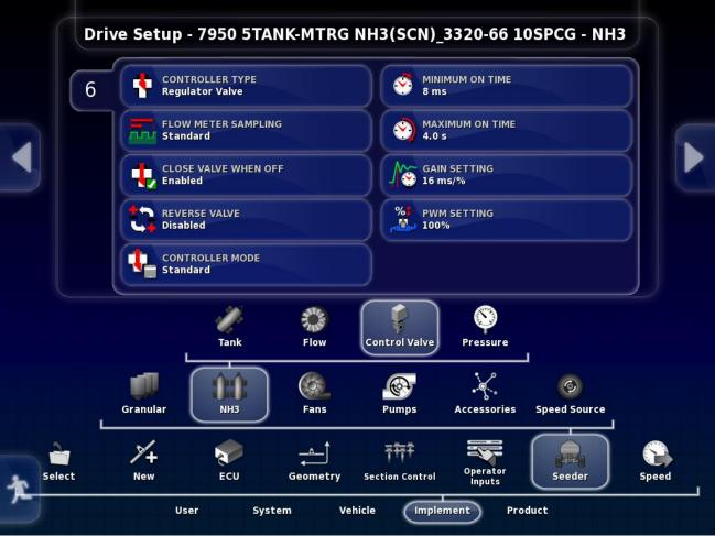
Select Implement/Seeder NH3 or Liquid/Control Valve then select Controller Type Regulator. If proportional was previously selected change to regulator then back to proportional after initial testing
