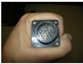
With your negative lead on pin 1 and the positive lead in pin 6 you should have 12 volts positive when you turn on section 1
