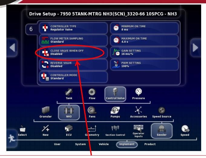
Close Valve if Tank is Off should be enabled if using a 4 wire Fast Valve and disabled if using a 2 Valve System (separate regulator and on/off valves).
