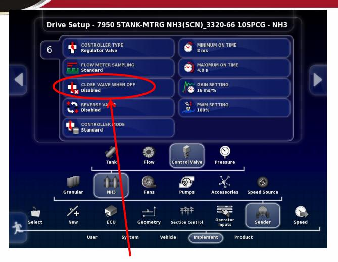
To test the 2 valve system you do not have the Close Valve When Off enabled so you will have to Enable Reverse Valve to see -12 volts when the negative lead is on pin 4 and the positive lead is on pin 3.
