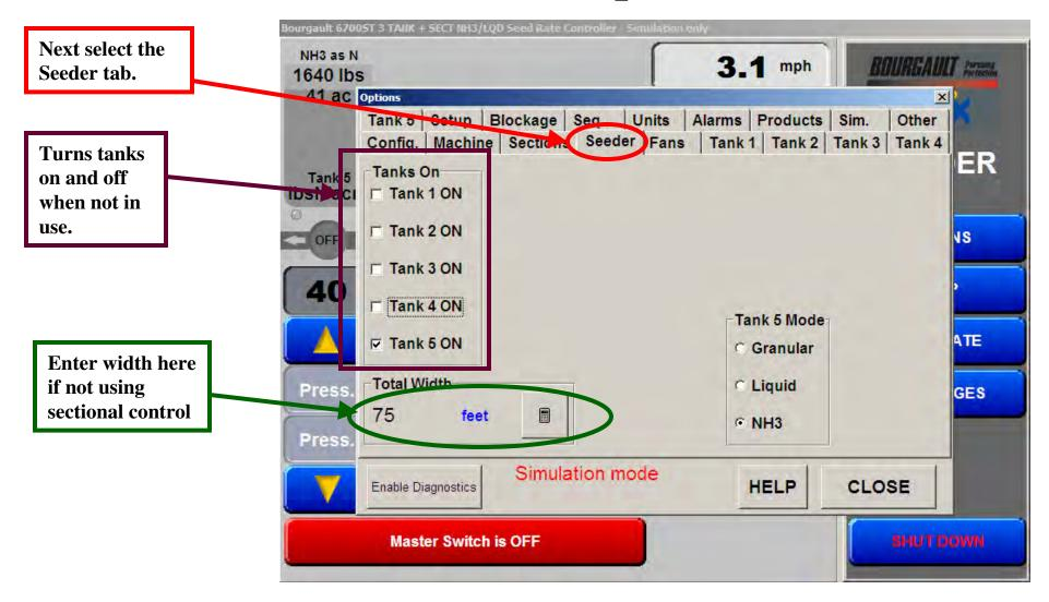
To run only the NH3 / Liquid turn granular tanks off.
