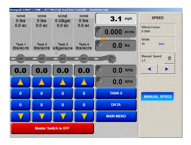
You must enter a manual speed to simulate movement, also remember to close the tank valve!
