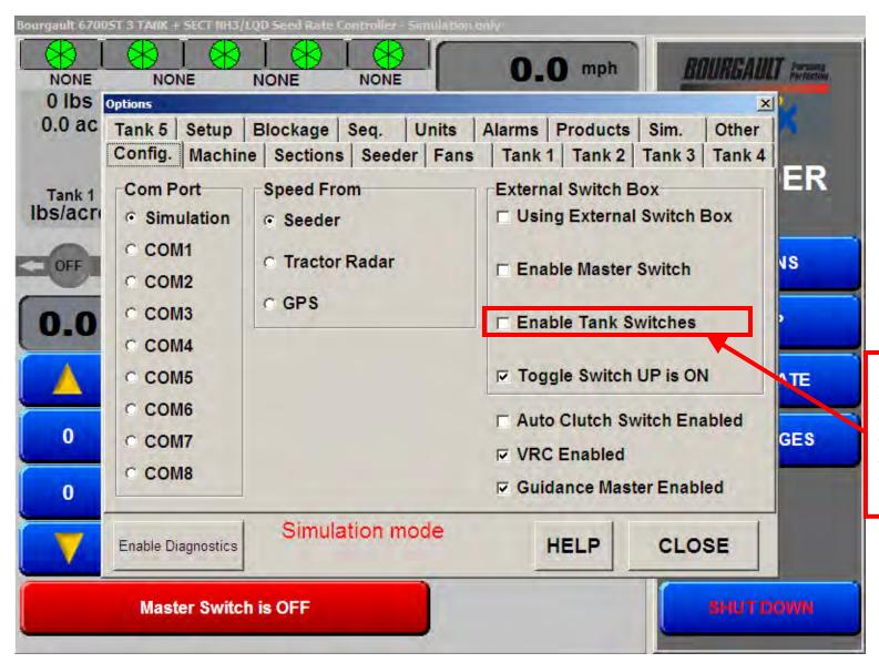
The external switch box has only 4 tank switches so this can only be selected if the Bourgault Air Seeder is metering out of 4 or less tanks. (NH3 / Liquid is Tank 5)
