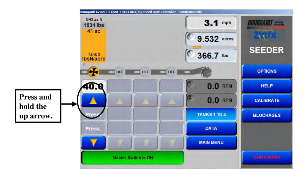
While holding the up arrow your volt meter should show positive 8 to 10 volts
