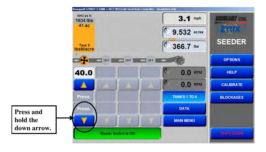
While holding the down arrow your volt meter should show negative 8 to 10 volts
