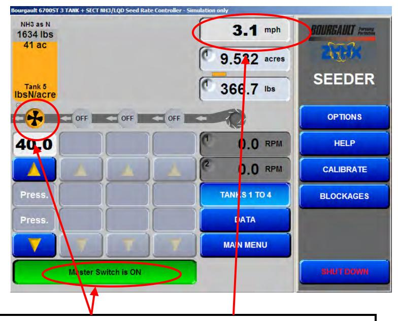
The master and tank clutches must be on as well as a manual ground speed.
