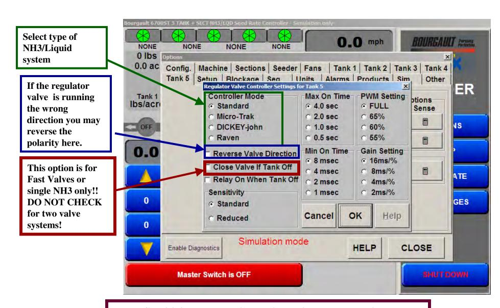
Leave Sensitivity, Max on time, Min on time, PWM settings and Gain settings at factory defaults unless advised by authorized technician!
