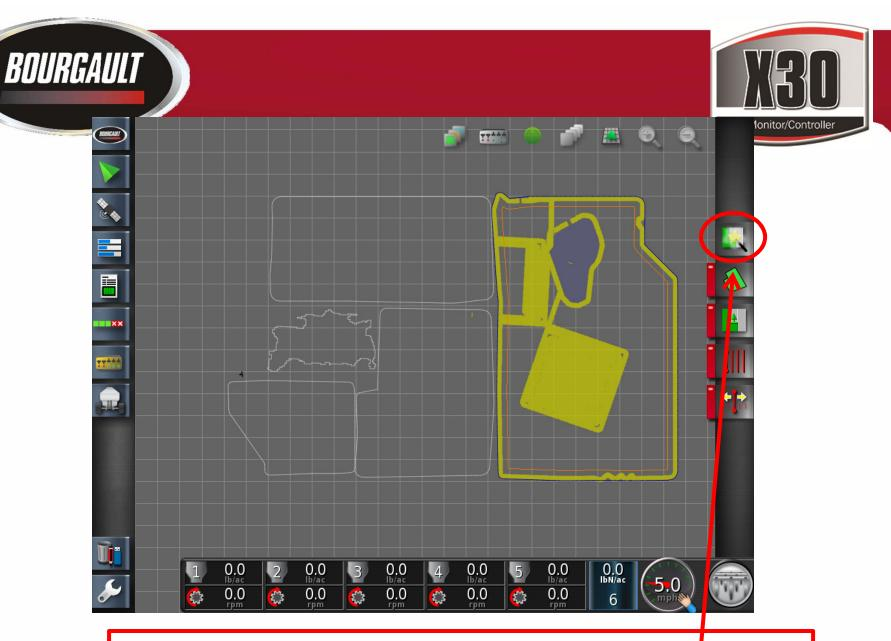
Exit the Setup section and enter the Guidance page. The Quick Start button is located at the top of the right hand menu.
