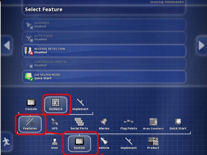
To enable Quick Start go to System/Features/Guidance
