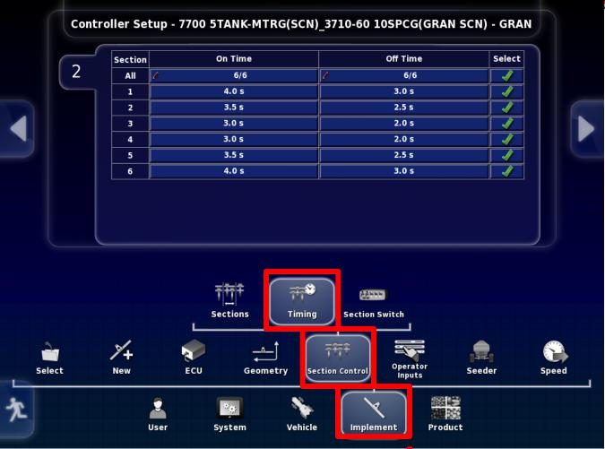
Enter the calculated ON and OFF times in Implement/Section Control/Timing
