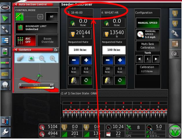
To complete the timing test you must have product in a tank directed to the openers and one directed to the MRB's if equipped.
