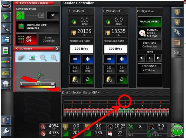
When the section is on press the section icon to turn it off then start timing once the dot turns red for each section and record the OFF time.
