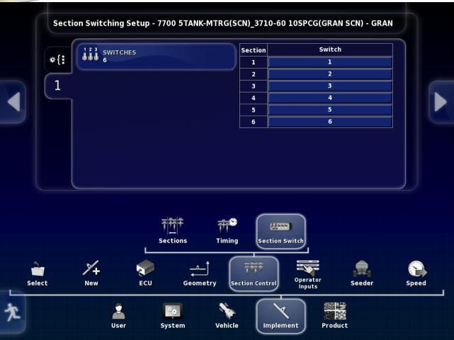
Verify that the X30 is set up with the correct number of sections to match the drill.
