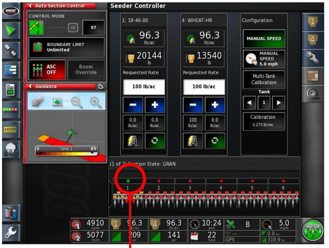
Select the each section switch one at a time and start timing once the dot turns green. Repeat this a few times to get and average ON time then record this number for entry.
