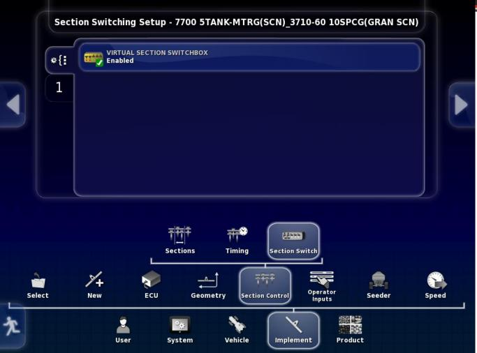
The virtual Section Switchbox should be enabled, go to Implement/Section Control/Section Switch.
