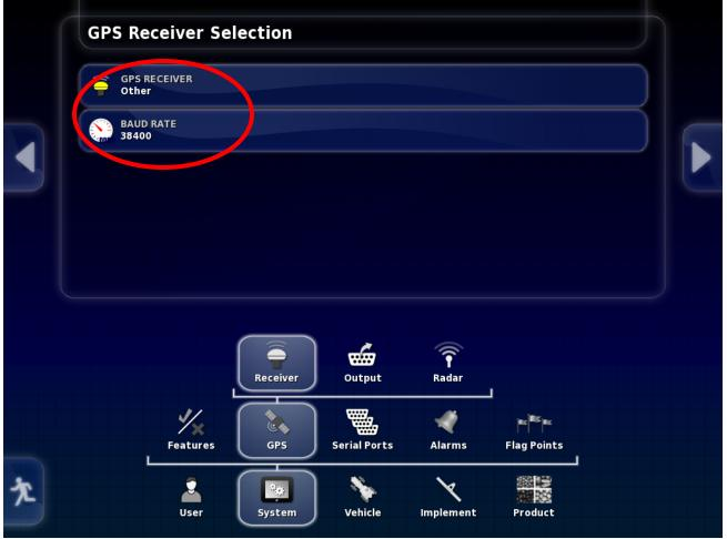
Set GPS RECEIVER to Other and BAUD RATE to match the Starfire 3000 output rate
