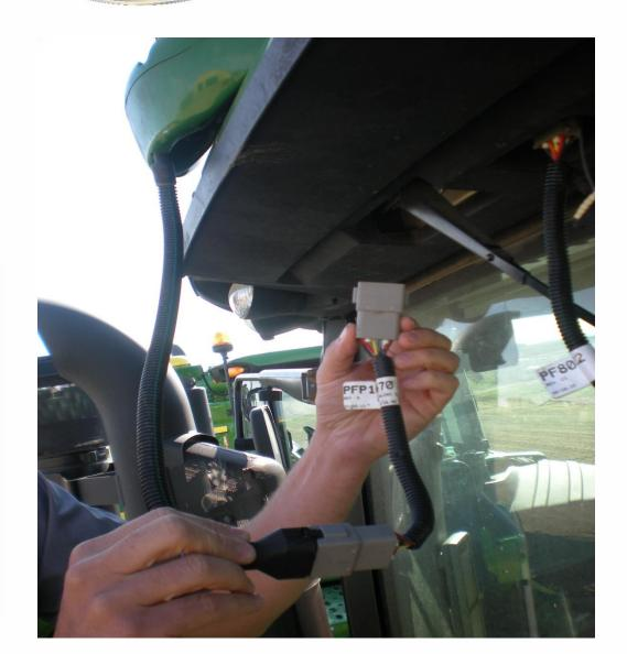
Connect the female/female PF10470 to the receiver cable that was unhooked from the tractor earlier.
