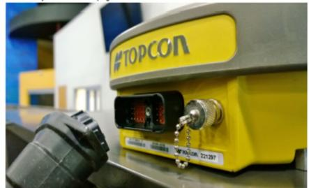
6. The screen will give you a warning that it is not communicating with the gps receiver. Again press the button beside the green check mark in the lower left hand corner. Within 30 seconds of pressing this button plug the gps receiver back in and the firmware will begin to load.
