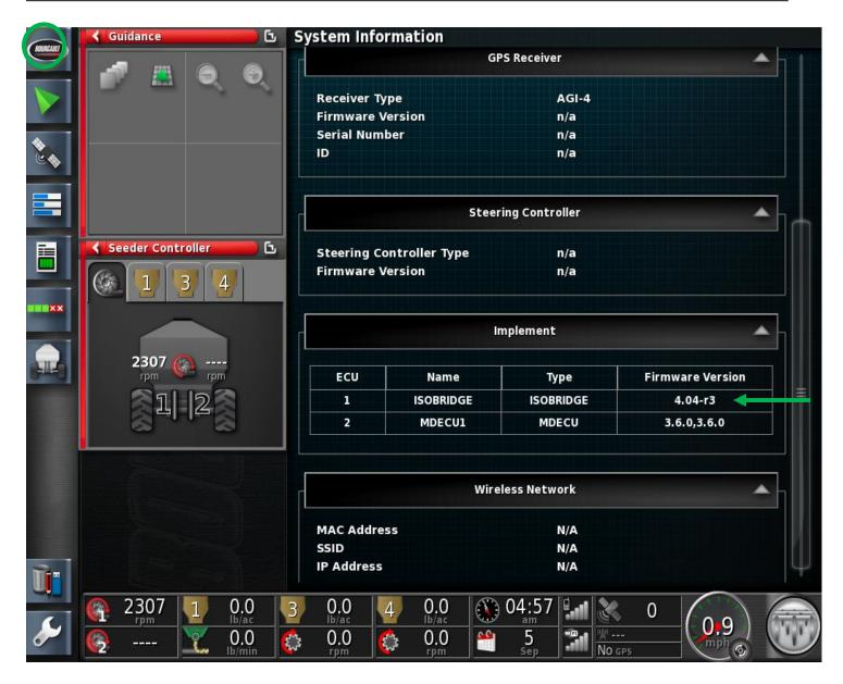
8. If monitor is hooked to the tank, the MDECU and SECU version will appear.
