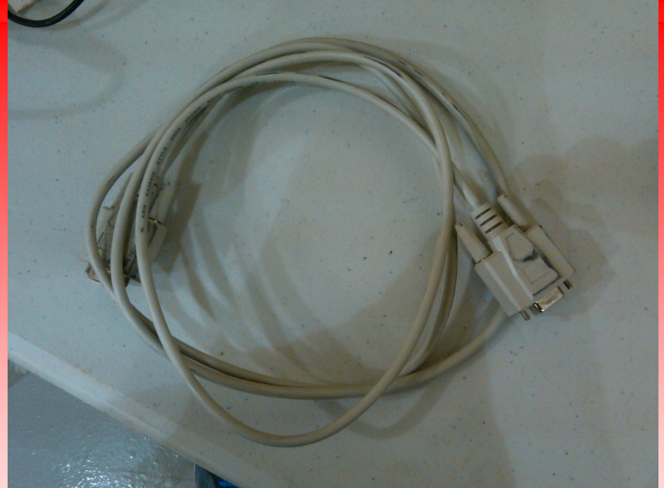
9 pin communication cable used to tie the monitor to the SRC interface
